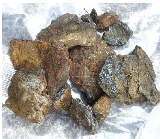
Figure 4: Photo of sample H909193 of semi-massive sulphide and gossan (20-30% oxidised pyrite and gossan) in mafic volcanic rock with assays returning 42.4 g/t Au.
