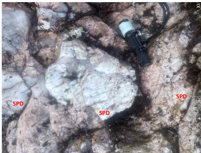
Figure 2 (top left): Photo of sample H909418 from Polaris. Photograph field of view contains 80% white to pinkish stained spodumene (SPD), 20% translucent quartz and feldspar. NB: UV light is 9cm for scale.
